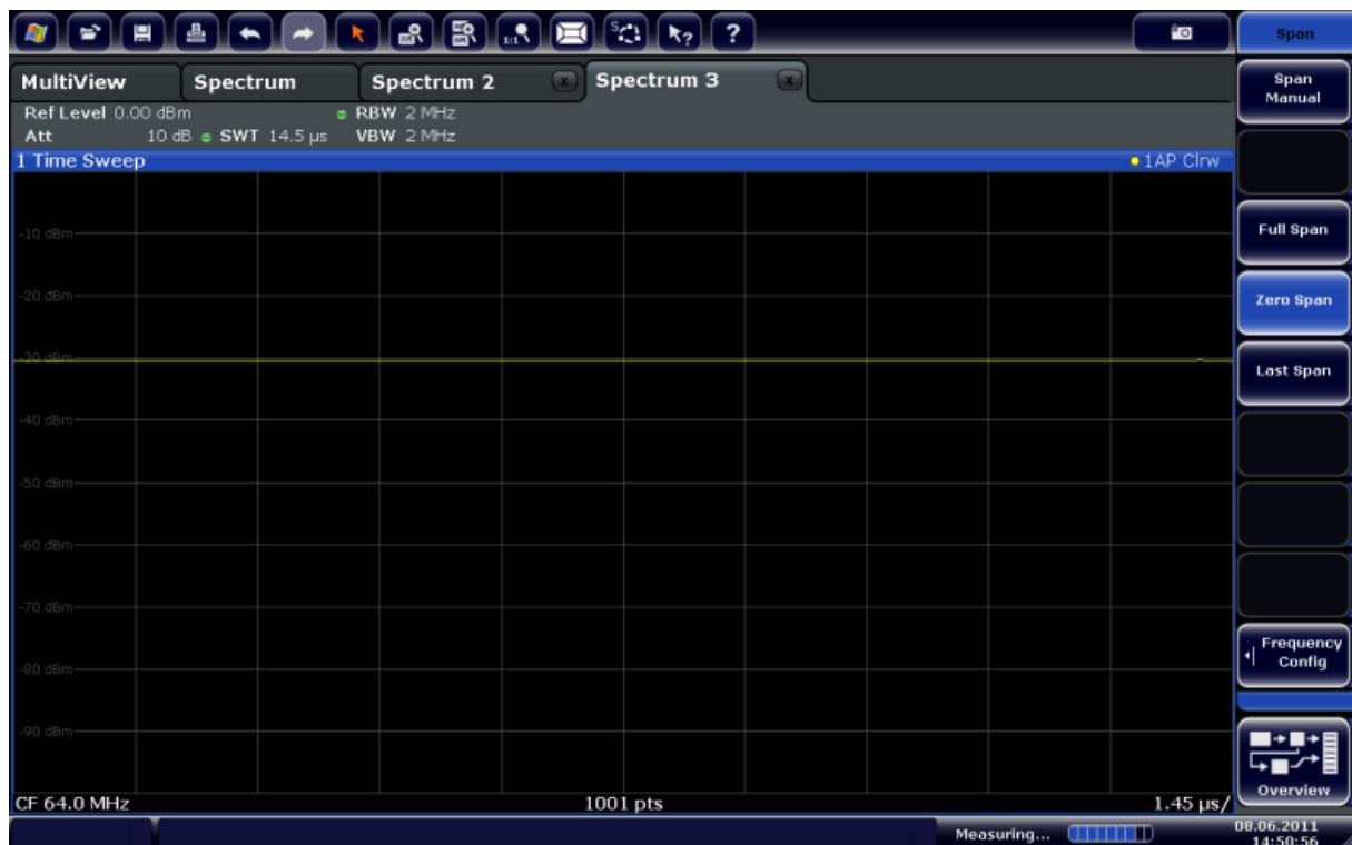
Fig. 4-7: Time domain display of the calibration signal
